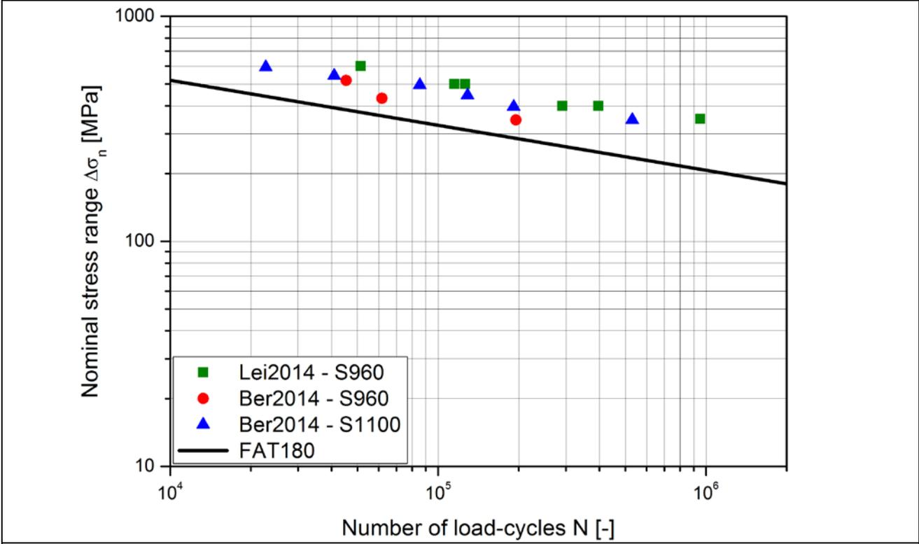
Figure 10 — Butt welds with  $950 < f_y$
