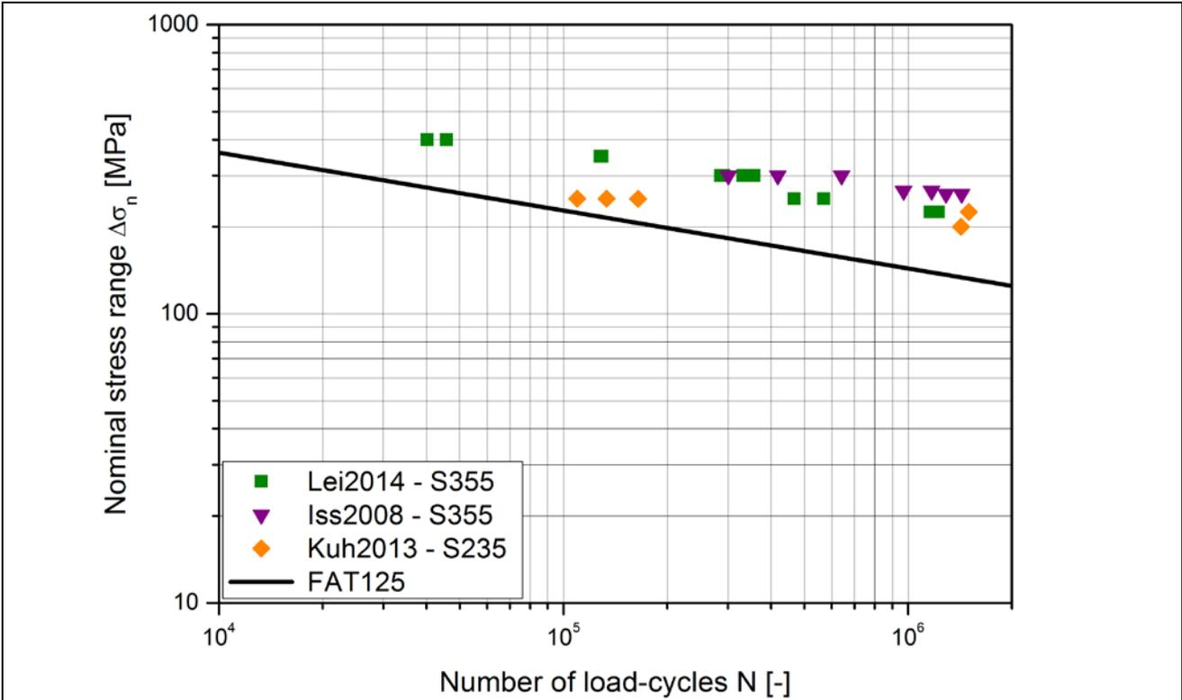
Figure 11 — Transverse welds with  $235 < f_y \leq 355$
