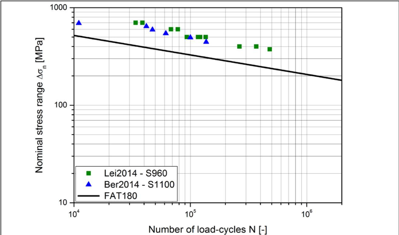
Figure 13 — Transverse welds with  $950 < f_y$
